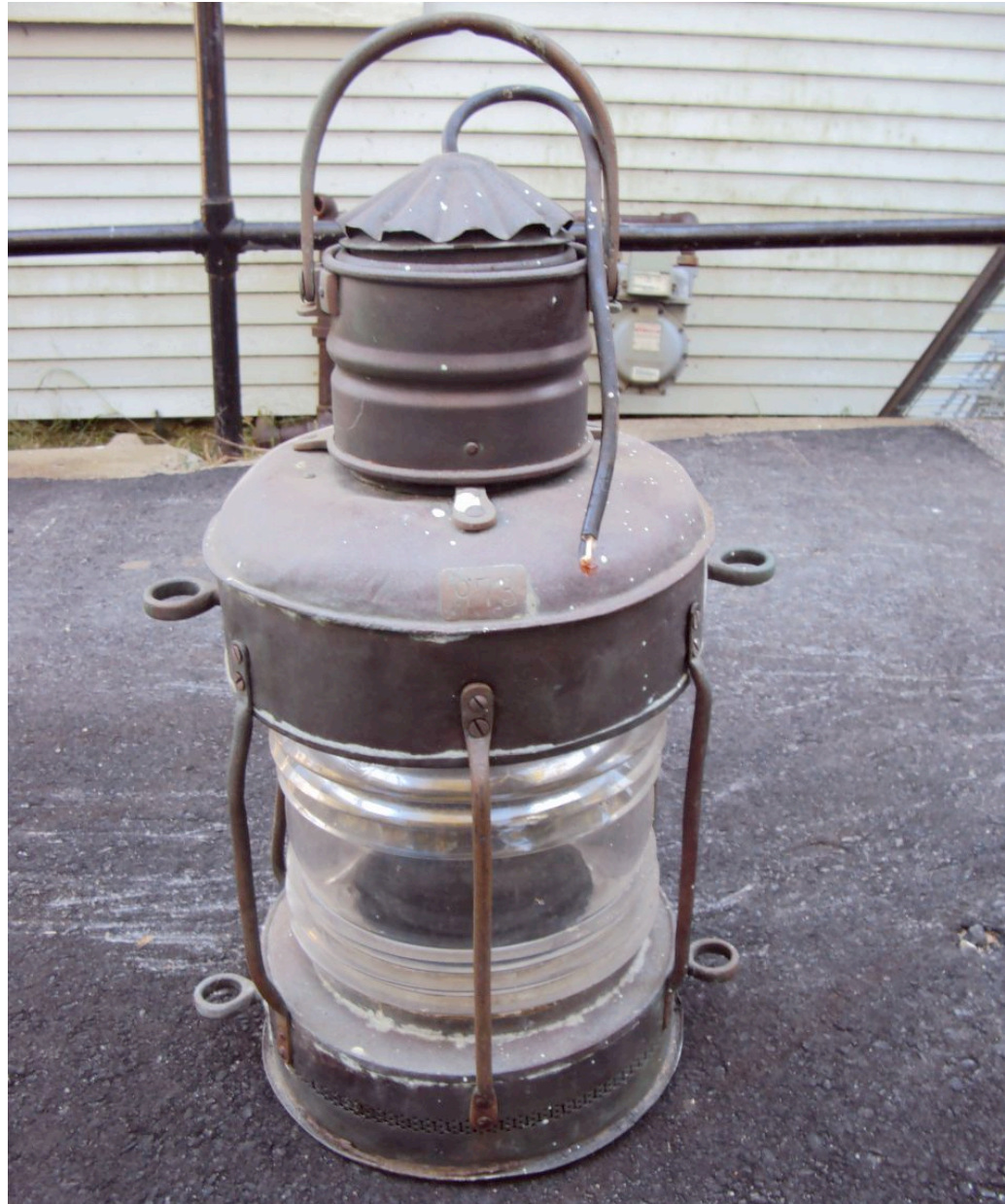
Sailing Ship's Anchor Lantern Used to Protect Ships at Night when Anchored in a Harbor
